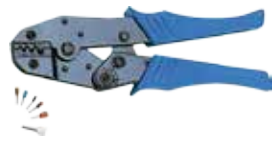
LY-2026(1307) CRIMPING CORD END TERMINALS 1: 0.5-0.75mm 2 2: 1.0mm 2 3: 1.5mm 2 4: 2.5mm 2 5: 4.0mm 2 6: 6.0mm 2
