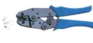
LY-2026(1322) CRIMPING NON-INSULATED TERMINALS 1: 22-16 AWG (1.25mm 2 ) 2: 16-14 AWG (2mm 2 ) 3: 12-10 AWG (5.5mm 2 ) 4: 8 AWG (8mm 2 )
