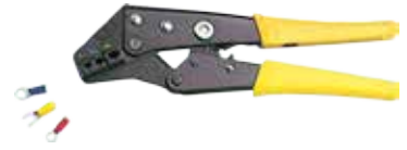
HRI-126J CRIMPING INSULATED TERMINALS 1. RED 22-16 AWG (1.25mm 2 ) 2. BLUE 16-14 AWG (2mm 2 ) 3. YELLOW 12-10AWG (5.5mm 2 )
